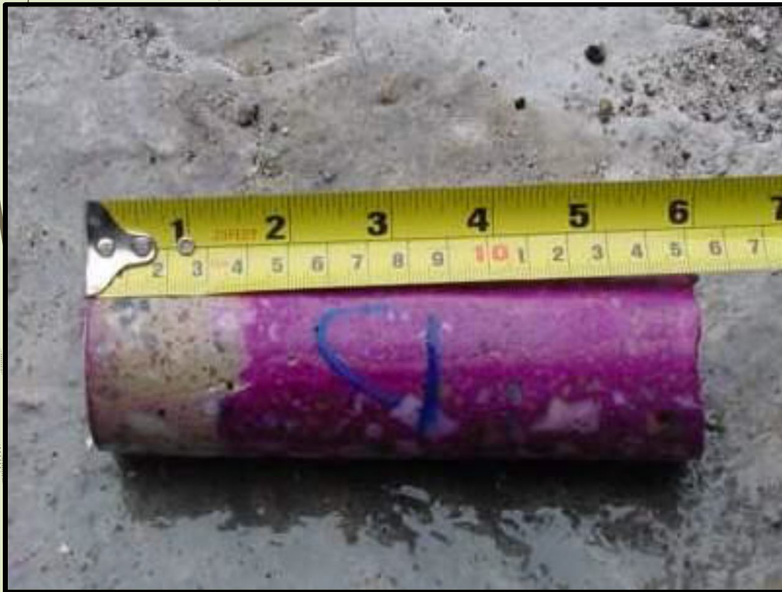
Measuring the carbonation depth of a core sample
