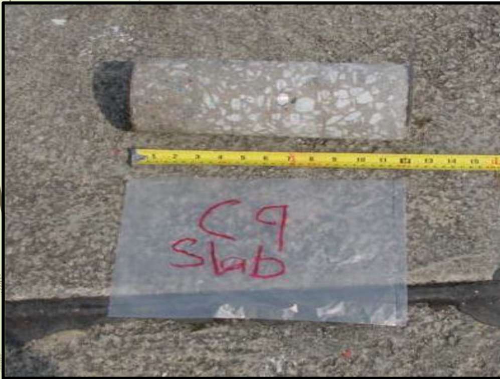
Core specimen ready for carbonation test
