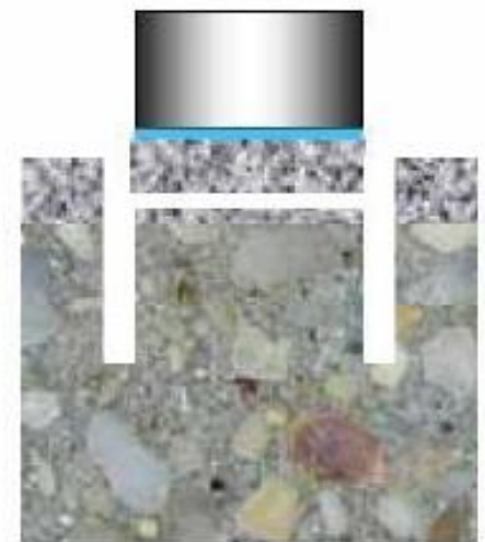
(c) Failure in overlay
