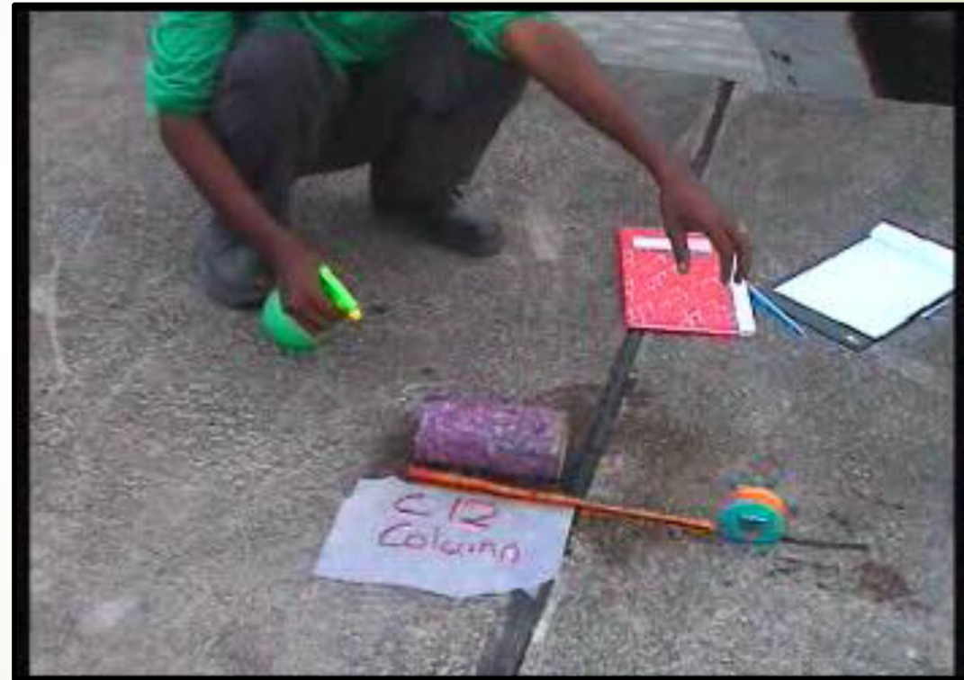
Spraying phenolphthalein solution on a core sample
