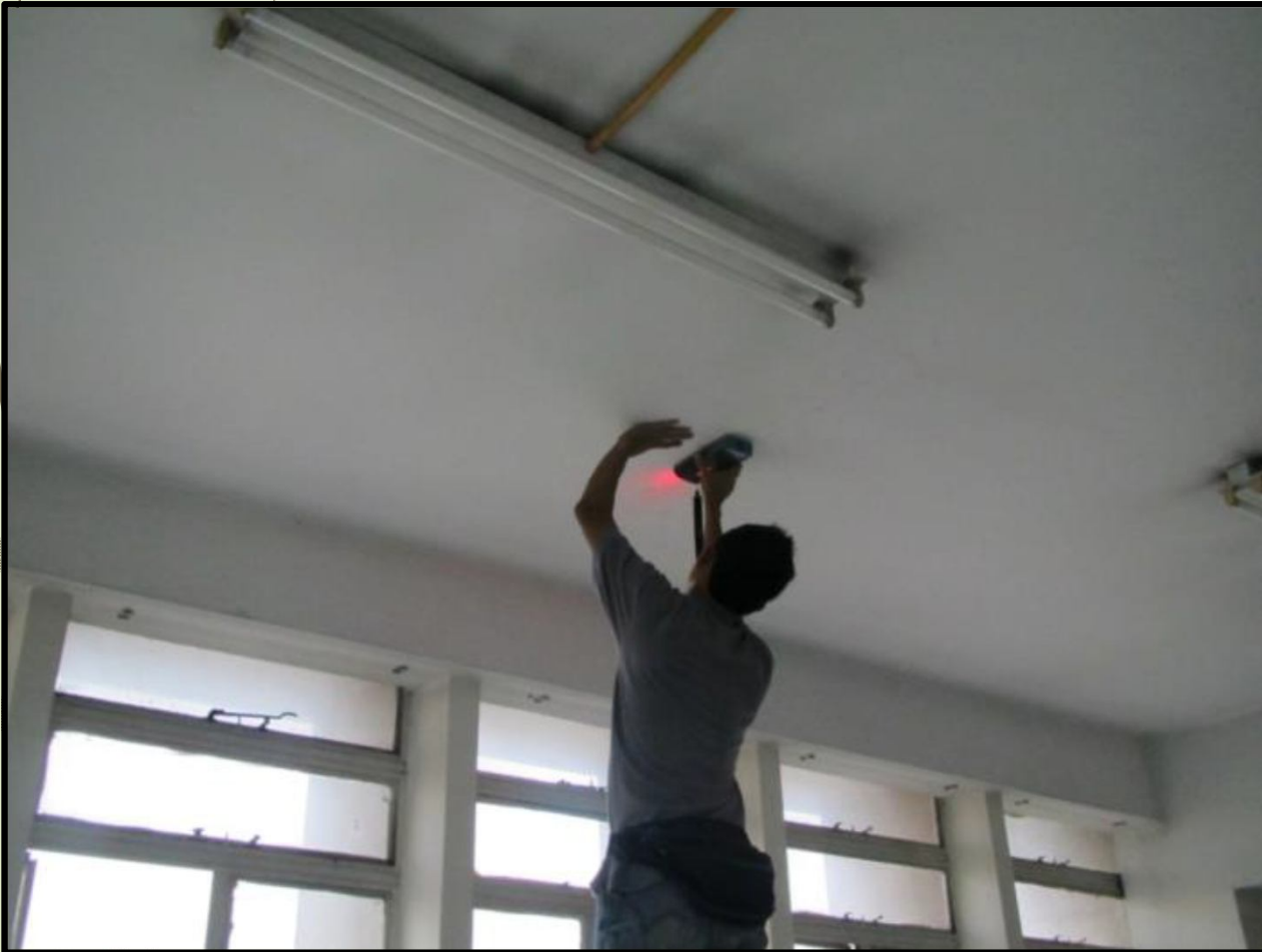
Scanning the rebar
