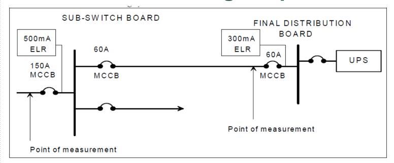
If the value of the neutral to earth voltage at Final DB is lower (or slightly) than value at SSB, this indicates that the high neutral to earth voltage originate at upstream.
