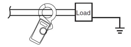
Leakage Current Measurements on the Single-Phase Systems
