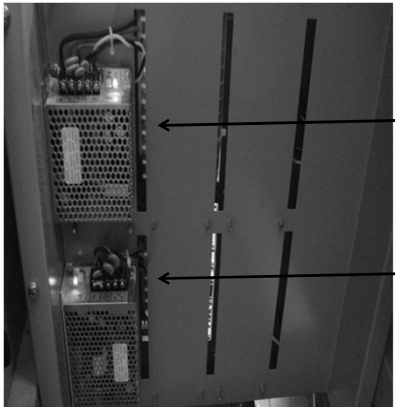
Power Supply Unit 110/220V: 5v (Yellow Cable)
