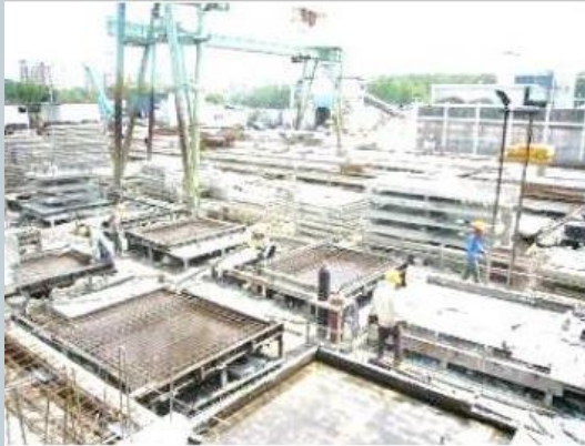
Conventional horizontal production using flat moulds
