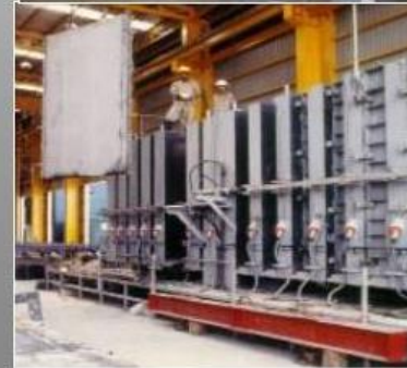
Vertical Production Using Battery Moulds
