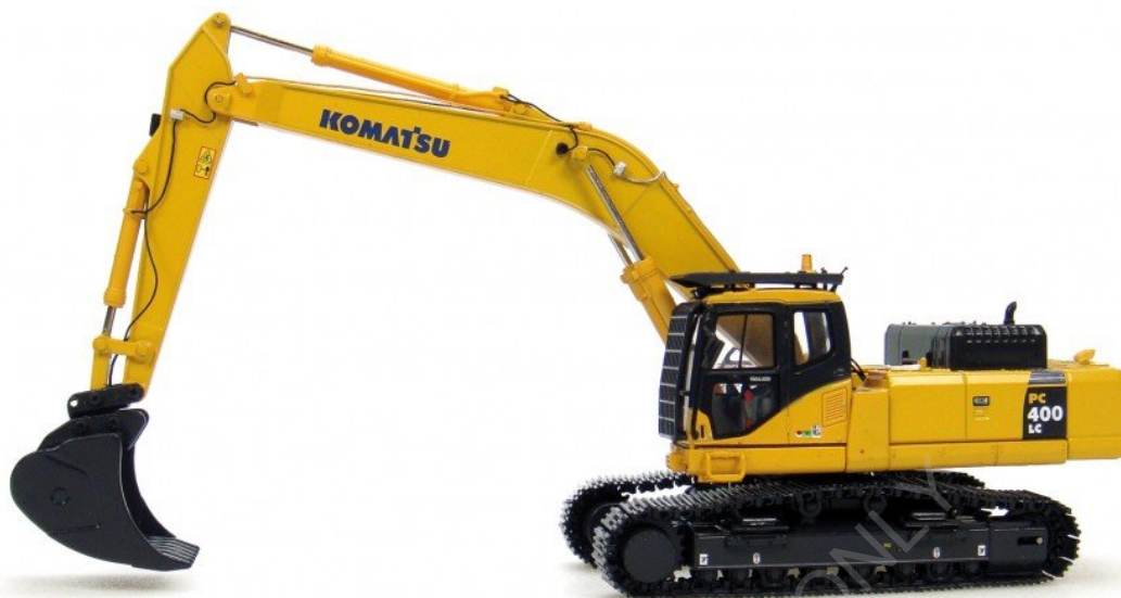
FIGURE 2.3: EXCAVATOR (SERIES 400) OF 41.4 TONNES AND 321 BHP (OR EQUIVALENT)
