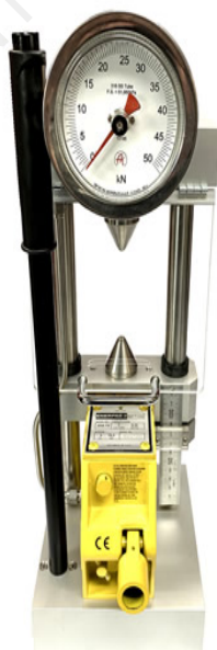
FIGURE 2.2: PORTABLE HYDRAULIC POINT LOAD TESTER WITH A PRESSURE-GAUGED READOUT FOR LOAD MONITORING (OR EQUIVALENT)
