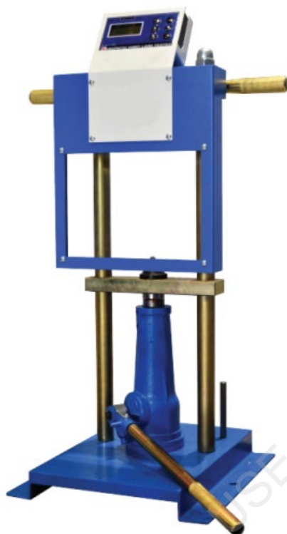
FIGURE 2.1: PORTABLE HYDRAULIC POINT LOAD TESTER WITH A STAIN-GAUGED LOAD CELL AND DIGITAL READOUT FOR LOAD MONITORING (OR EQUIVALENT)
