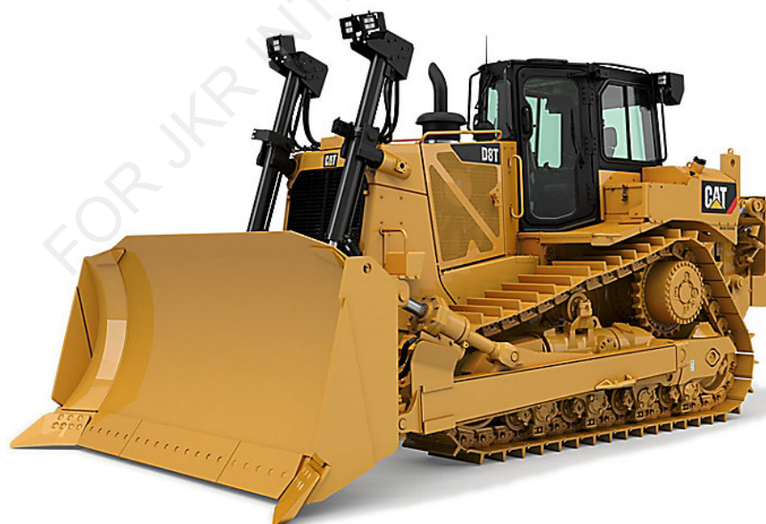
FIGURE 2.4: TRACK-TYPE OF TRACTOR (D8 DOZER) OF 37 TONNES AND 303 BHP (OR EQUIVALENT)
