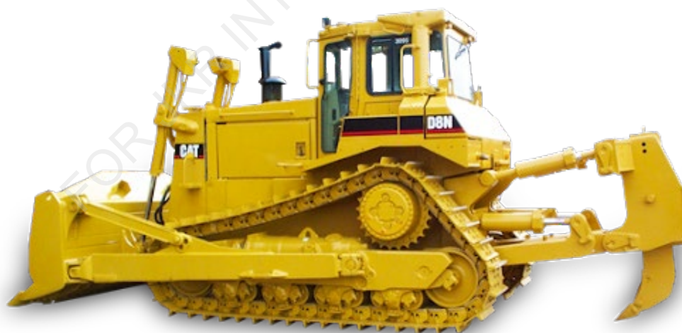
FIGURE 2.6: TRACK-TYPE OF TRACTOR (DOZER) ATTACHED WITH SINGLE SHANK RIPPING EQUIPMENT (BULLDOZER RIPPER) (OR EQUIVALENT)
