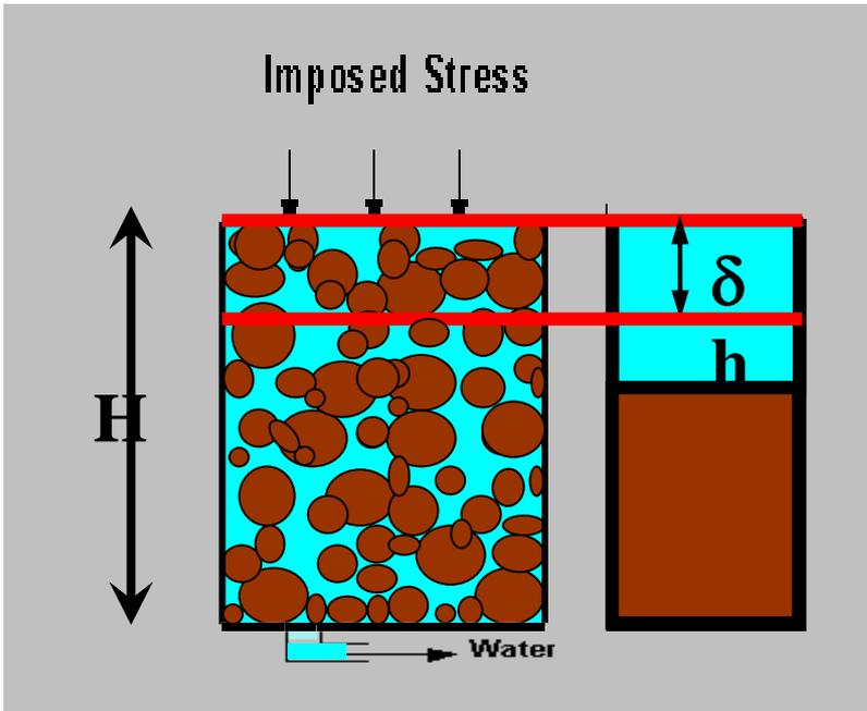
**Drainage of excess pore water pressure** Induced by increase in stress
