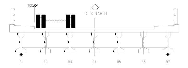
POSITION OF STRAIN GAUGES AND PRECISE LEVEL AT PIER 1
