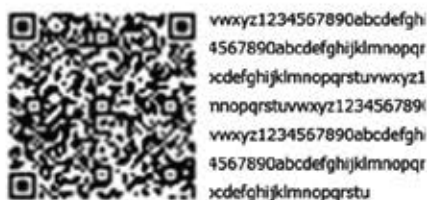
Figure 1: Capacity of a QR code that encodes 300 alphanumeric characters
