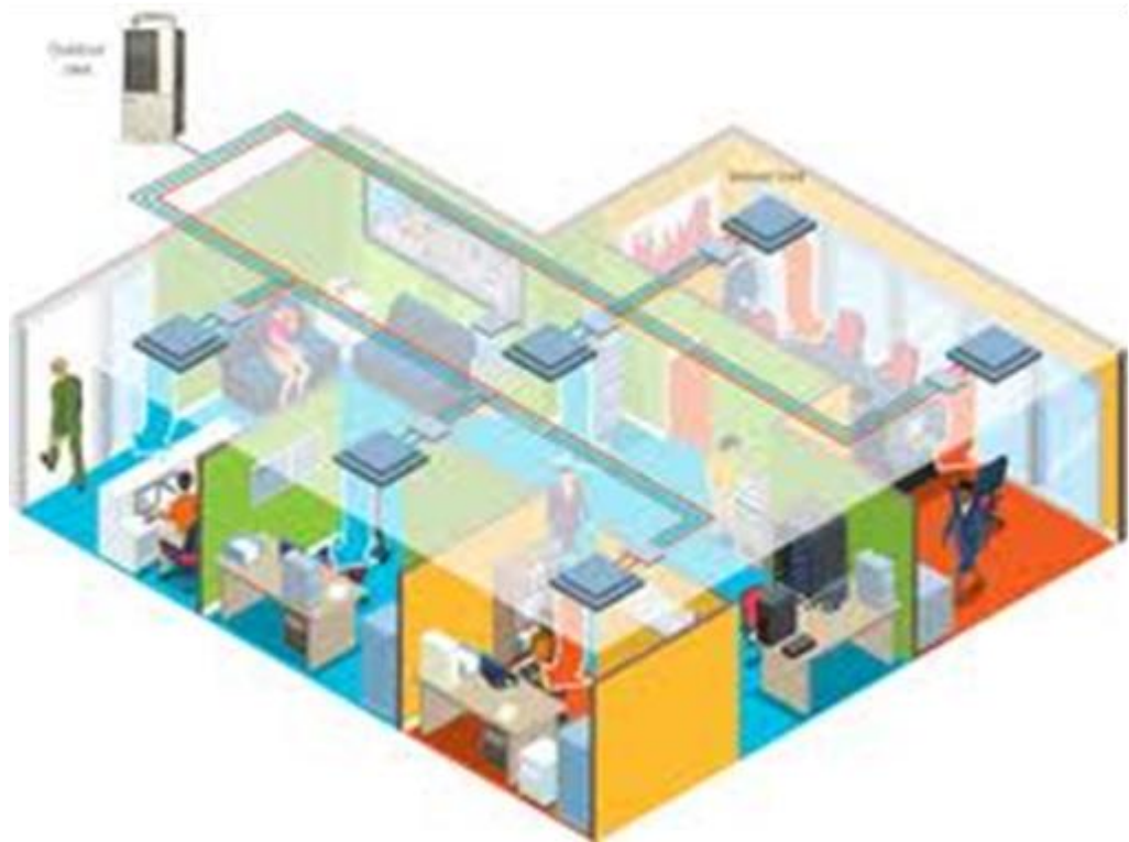
Figure 4.2 A typical layout of VRF system
