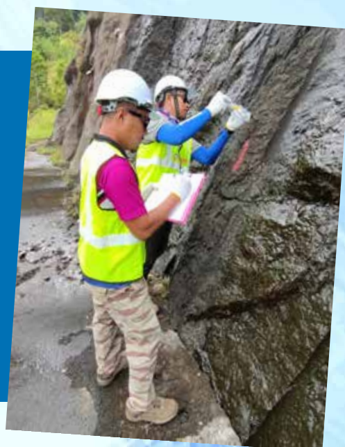
Figure 2: The Schmidt hammer N-type used
