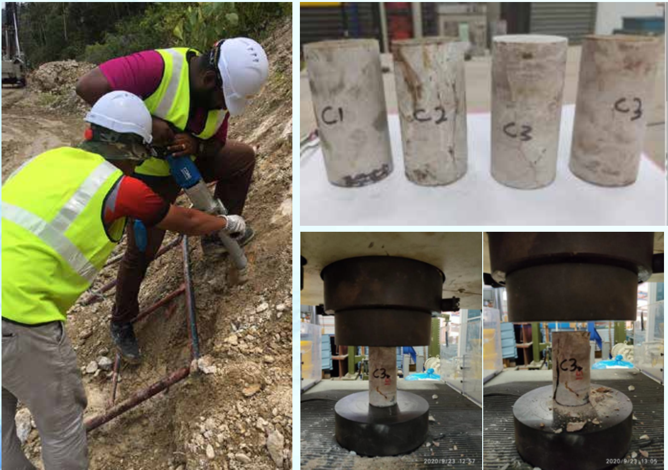
Figure 3: Rock coring at field and UCS laboratory testing
