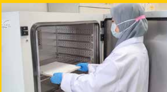
Figure 3: Conditioning sample in climate chamber
