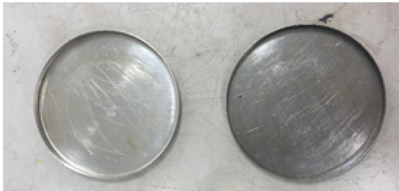
Pan, aluminium atau stainless steel, bergaris pusat 140 mm, tinggi 10 mm. Tebal aluminium 0.76 mm, tebal stainless steel 0.64 mm.
