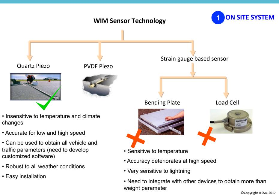
Quartz sensor was selected as a main sensor to produce traffic and vehicular data
