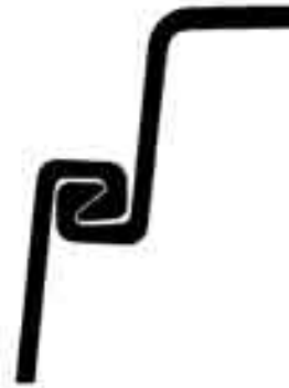
Figure 2-19 Larssen Type Interlock
