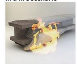
Steel protected with intumescent coating in a fire scenario
