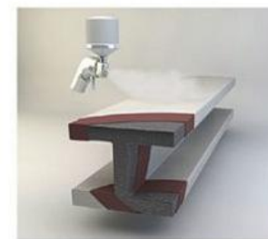
Steel protected with intumescent coating
