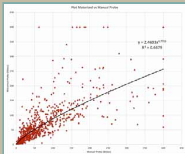
Figure 5: Plot Between Motorized and Manual Probe for Cohesive Soil
