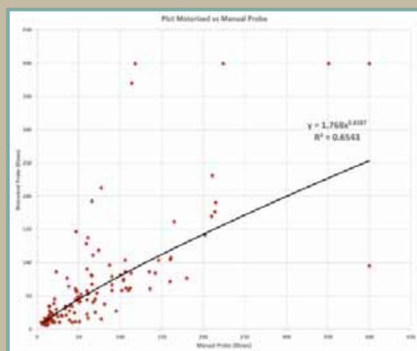
Figure 6: Plot Between Motorized and Manual Probe for Cohesionless Soil
