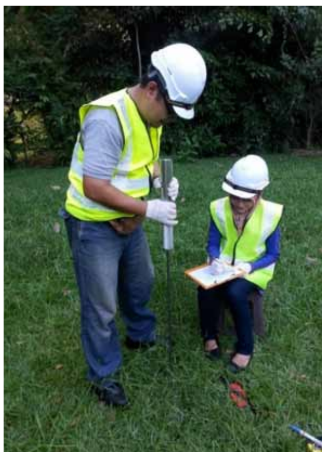
Figure 2: Manual Probe Test (courtesy of Eyda Mahasan)
