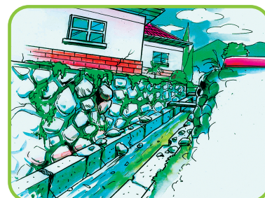
4. Bulging ground appears at the base of a slope or retaining wall.
