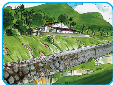
2. Water breaks through the ground surface in a new location near a slope.
