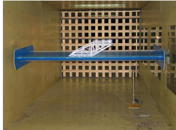
Figure 27 – Sutong Bridge Section Model Wind Tunnel Testing
