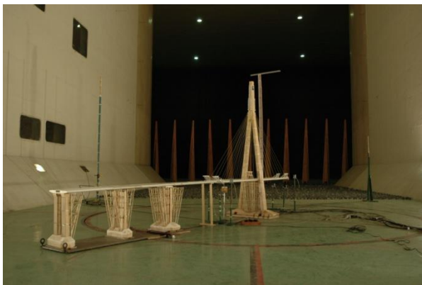
Figure 26 – Sutong Bridge Aeroelastic Bridge Model Wind Tunnel Testing
