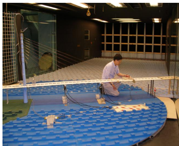
Figure 16 – Stonecutters Bridge Aeroelastic Bridge Model in the Wind Tunnel
