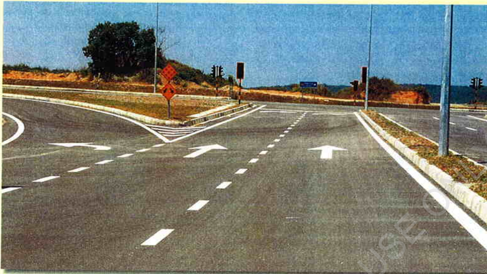
Photo 10 The visibility of the right hand primary traffic signal here is impaired by positioning the light pole in front of it. Note also the lack of prominence and legibility of the traffic sign on the far side of the road.
