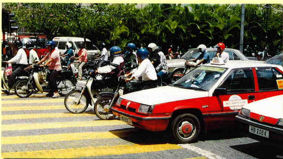
Positioning the signal pole too far ahead of the 'stop' line results in motorcycles, and sometimes cars, encroaching into the pedestrian cross-walk.
