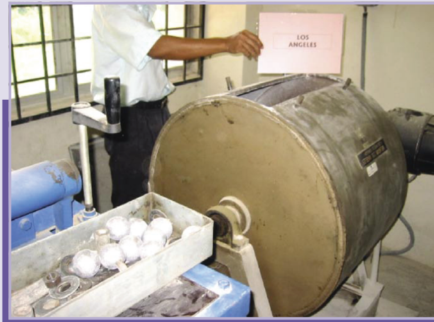
Drum lelasan Los Angeles (Los Angeles abrasion drum).
