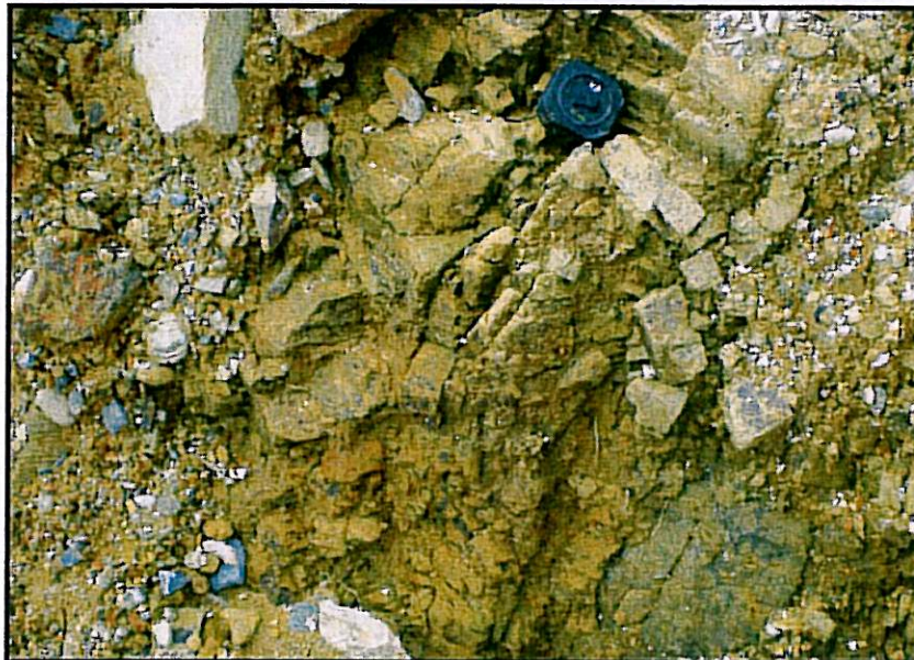
Plate 1D: Residual soil of gravelly silt and sand at the
