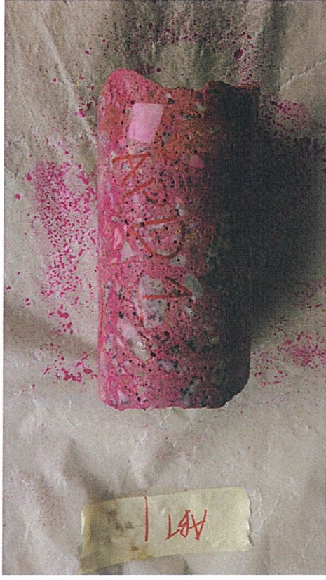
Carbonation Test to Concrete Core extracted from Abutment 1.
