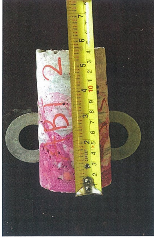
Picture 8 - Carbonation Test to sample from Abutment 2.
