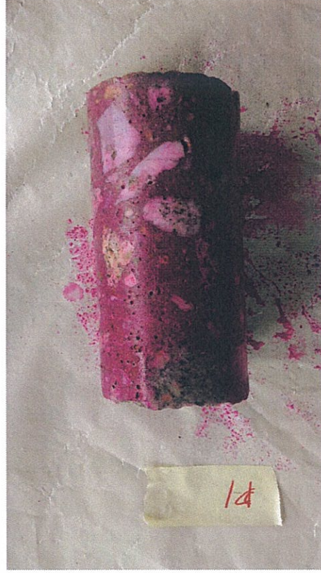
Carbonation Test to Concrete Core extracted from Pier 1.
