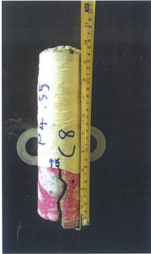
Picture 10 - Carbonation Test to sample from Pier 4.
