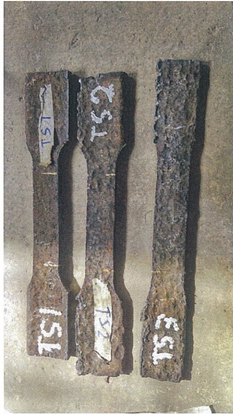
Picture 10 - The prepared Steel Coupons (Before)
