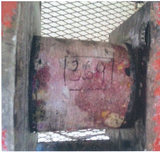
The prepared Concrete Core extracted from Pier 1.
