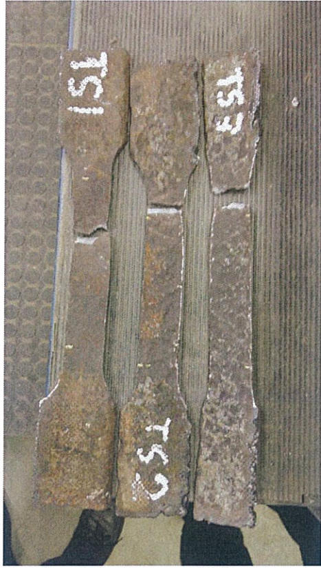
Picture 11 - The tested Steel Coupons (After).
