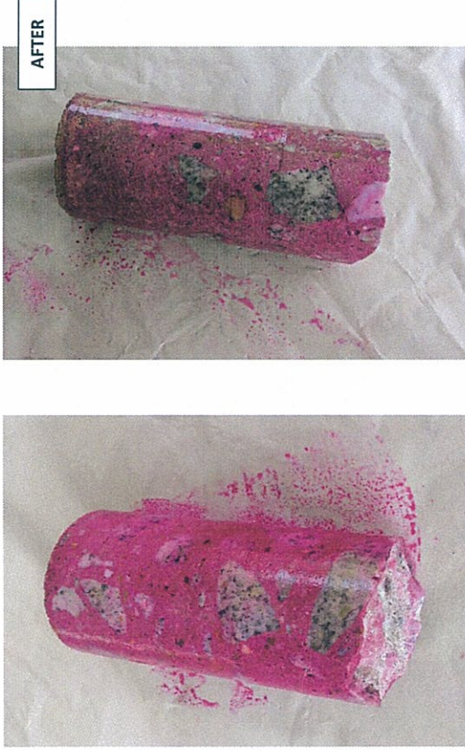
Carbonation Test to Concrete Cores extracted from Pier 4 (Left) and Pier 5 (Right).
