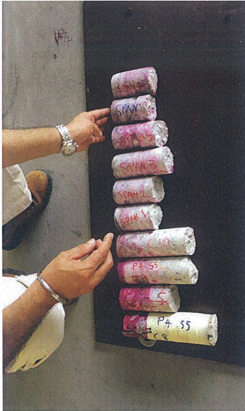
Picture 1 - Carbonation Samples Overview. (68 mm \phi )
