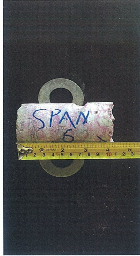
Picture 6 - Carbonation Test to sample from Span 6 Slab.
