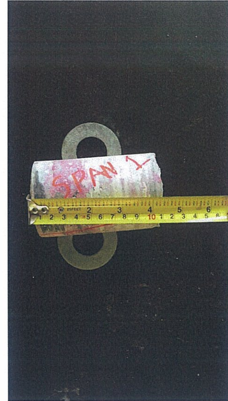
Picture 2 - Carbonation Test to sample from Span 1 Slab.
