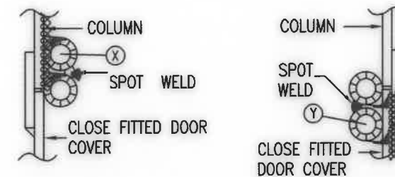
DETAIL 3: DOUBLE SLOT HINGED RIVETED TO COLUMN
