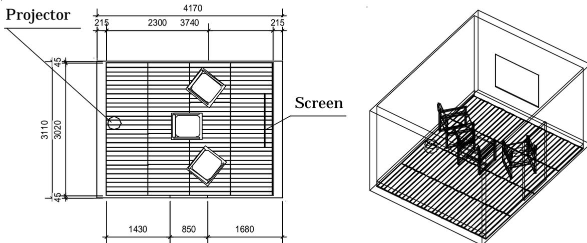
Figure 1 Details of the Artificial Weather Chamber
