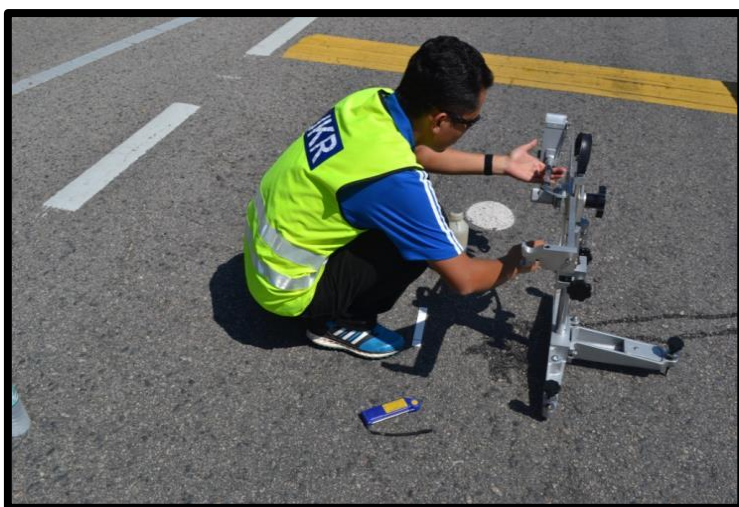
Picture 2: Skid Resistance Values Are Measured using British Pendulum Skid Tester. The test is conducted based on ASTM E303-87.
