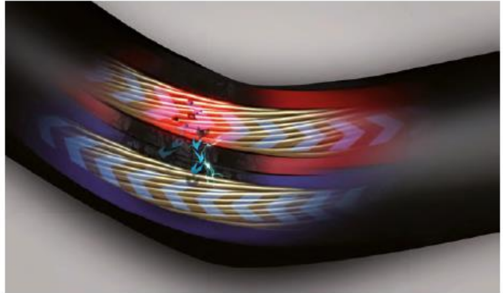
Fig. F77: Illustration of a resistive short circuit
