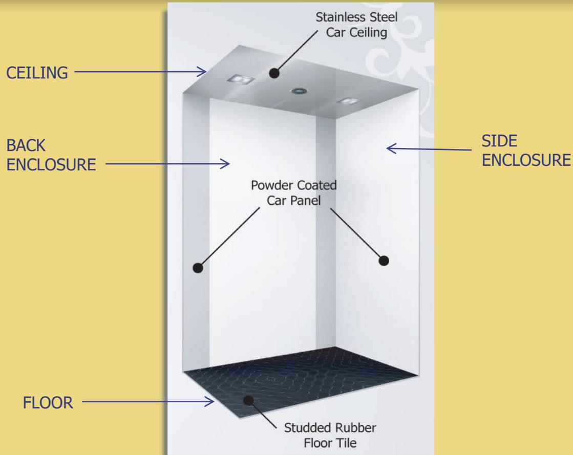
**Car platform of each passenger lift shall consist of a structural steel frame fitted with sufficient layers of hardwood flooring. Car platform shall be mounted on thick rubber pads supported by an auxiliary steel frame fastened to the car frame and the lift cab shall be bolted to the car platform without direct connection to the car frame. The car platform shall be equipped with a metal threshold plate, and the underside of the car platform shall be fireproofed with a steel sheet covering.**
