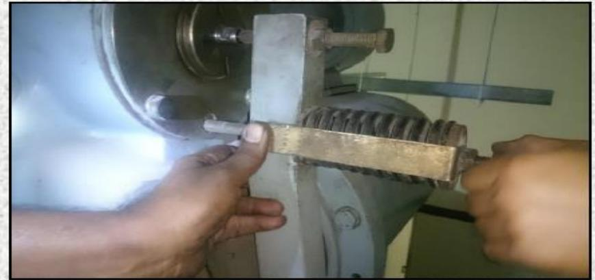
Brake system shall be of spring operated. The brake shoe shall be of double stroke type.
