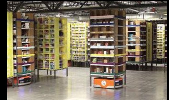
A Kiva robot carries a rack of merchandise across a storage area at the Amazon Fulfillment Centre.
