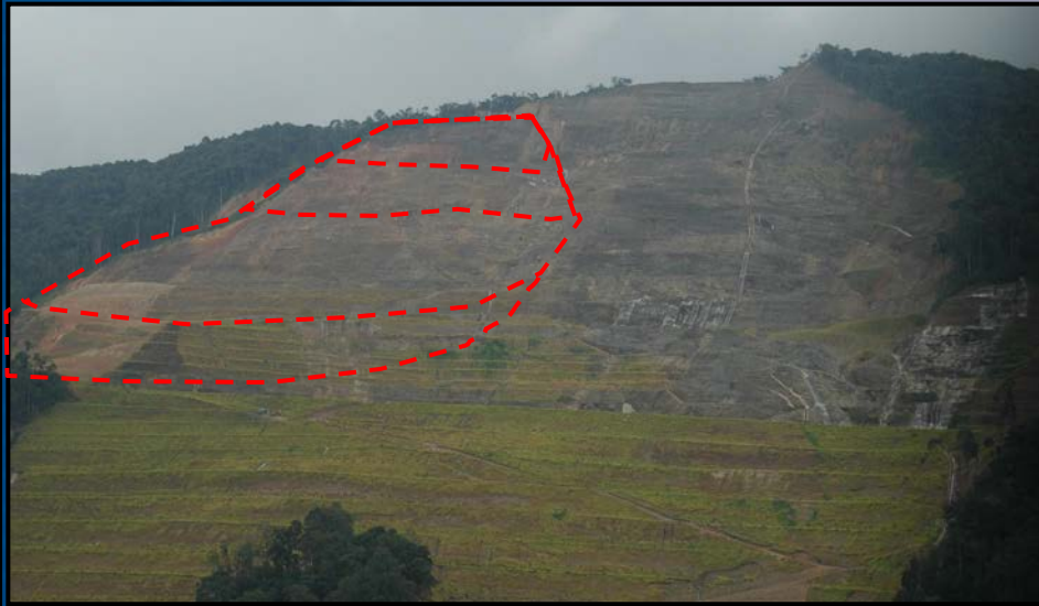
Field-sketch to show the approximate extend of the moving blocks within the major failure
