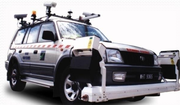
Surface Condition Survey
