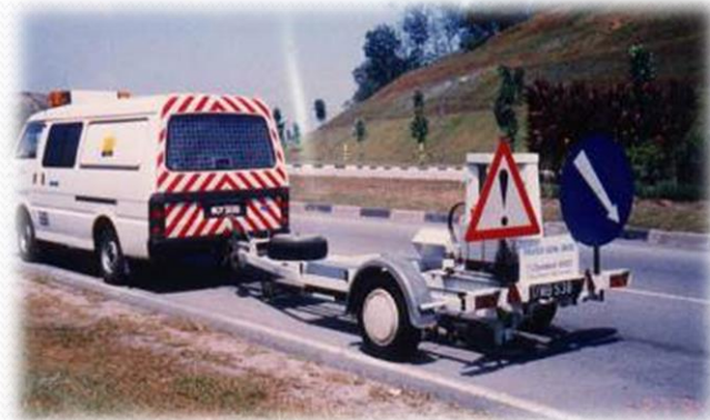
Deflection Test (Falling Weight Deflectometer)
