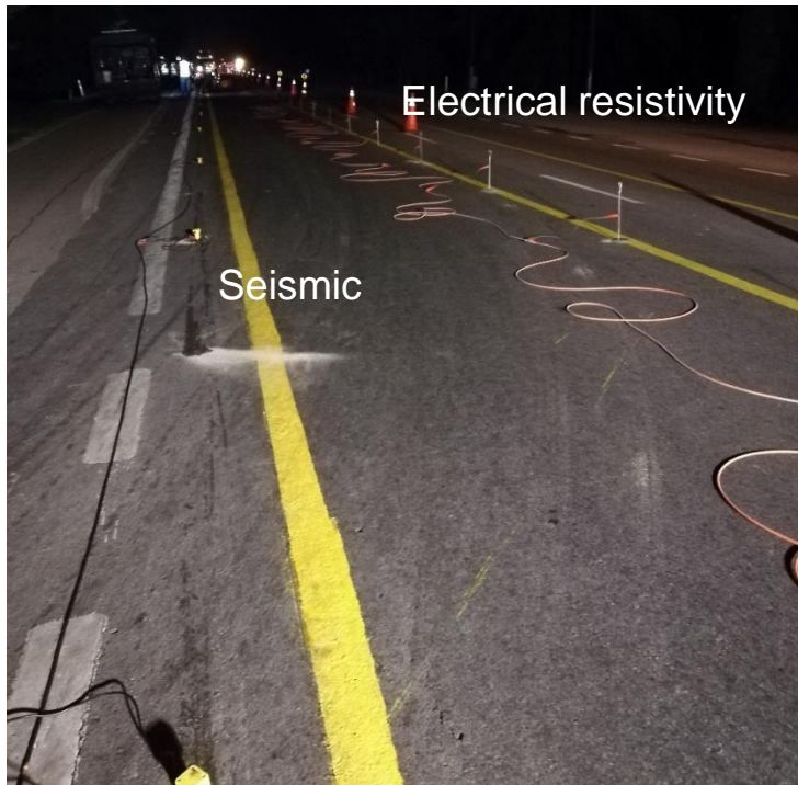
Setting of electrical resistivity and seismic at the site.
