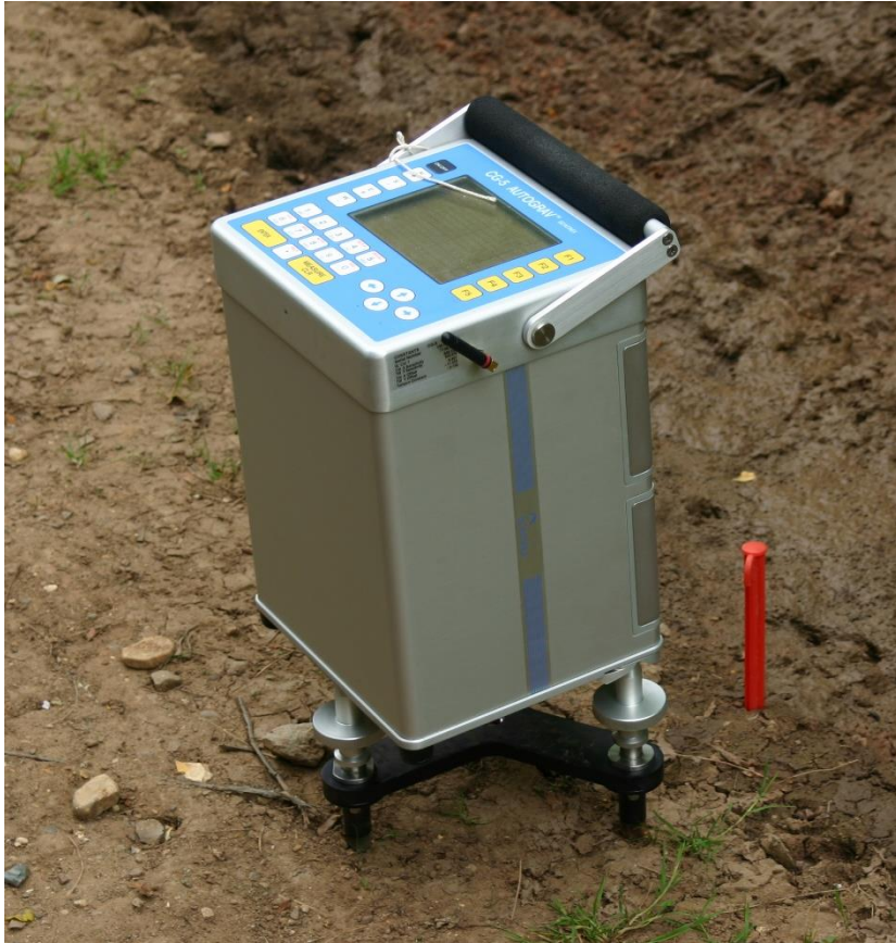
Equipment for gravity measurement known as gravity meter
