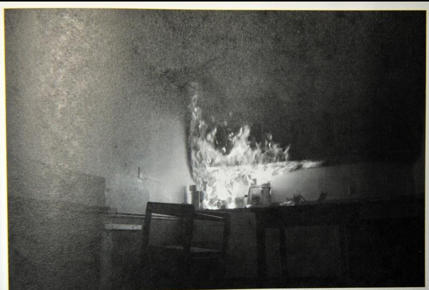
FIGURE 7.8B ♦ Fire spreads into cabinets. Plume entering air return grille in suspended ceiling. Courtesy of Jamie Novak, Novak Investigations.
