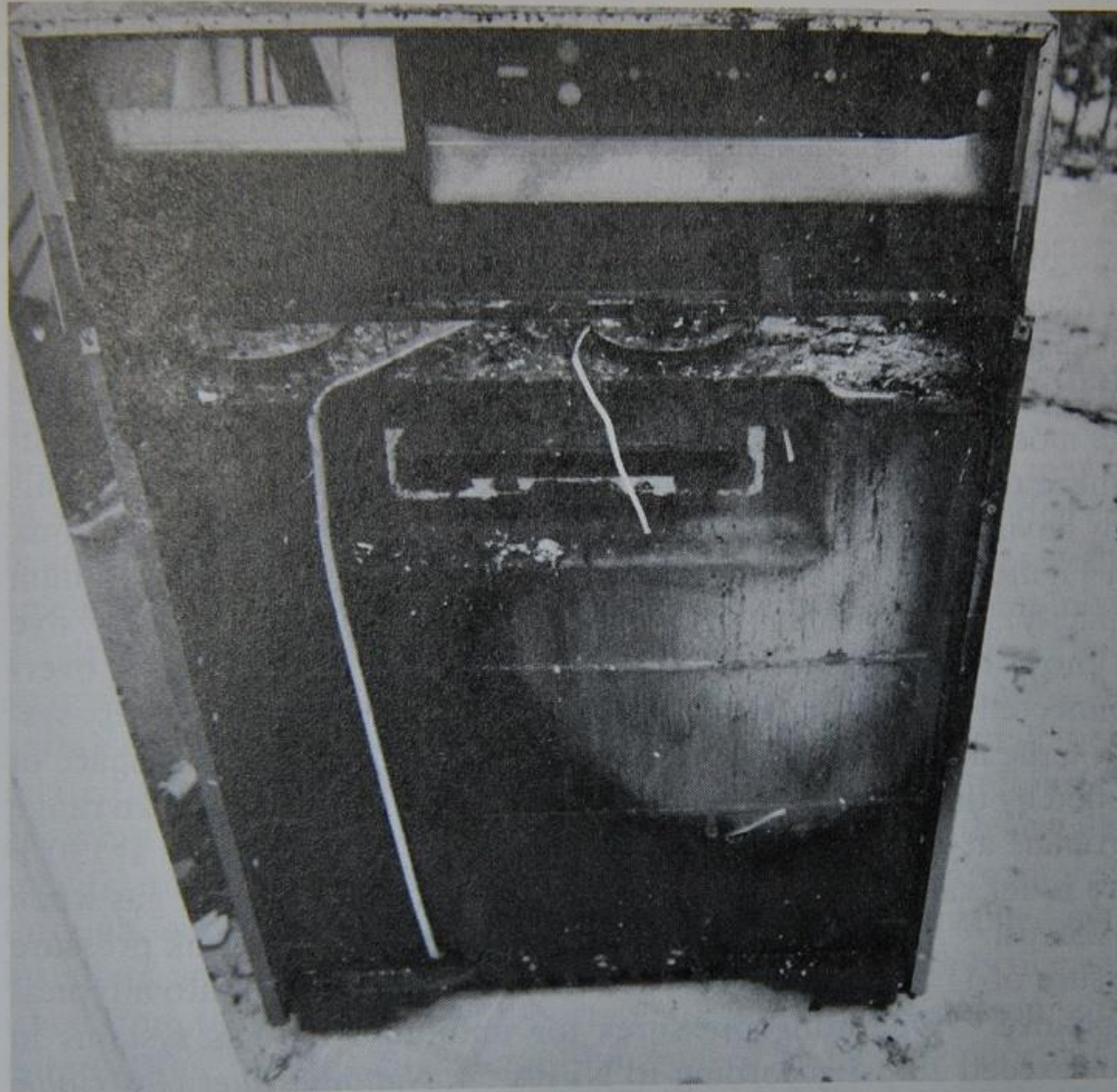
FIGURE 4.13B ♦ Plume damage (clean burn) on the back of the stove from the same gas plume. (The stove had been moved away from the wall prior to fire.) Courtesy of Det. Richard Edwards, Los Angeles County Sheriff's Department, Whittier, CA.
