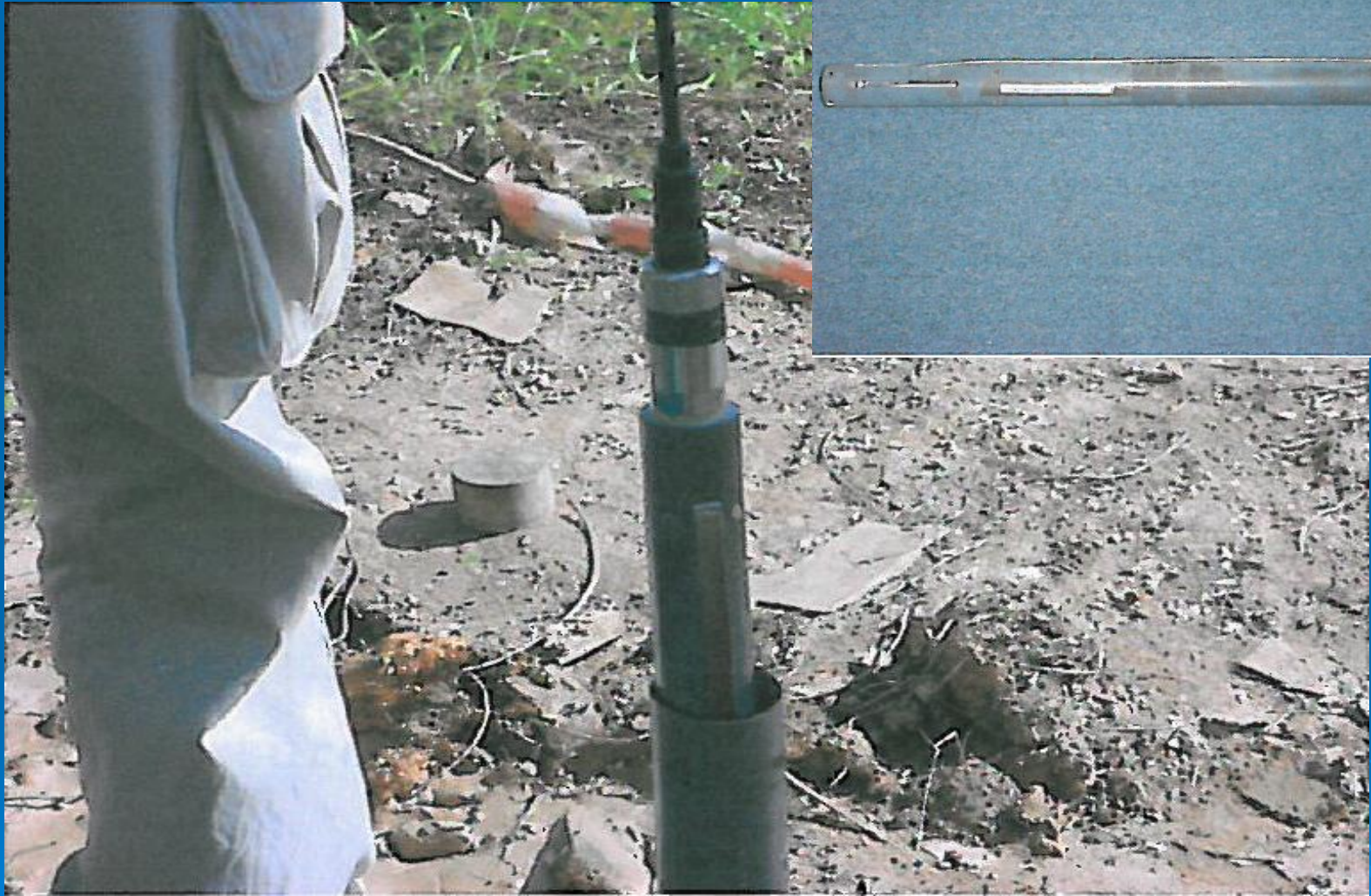
Lowering of Hydrophone into PVC Borehole
