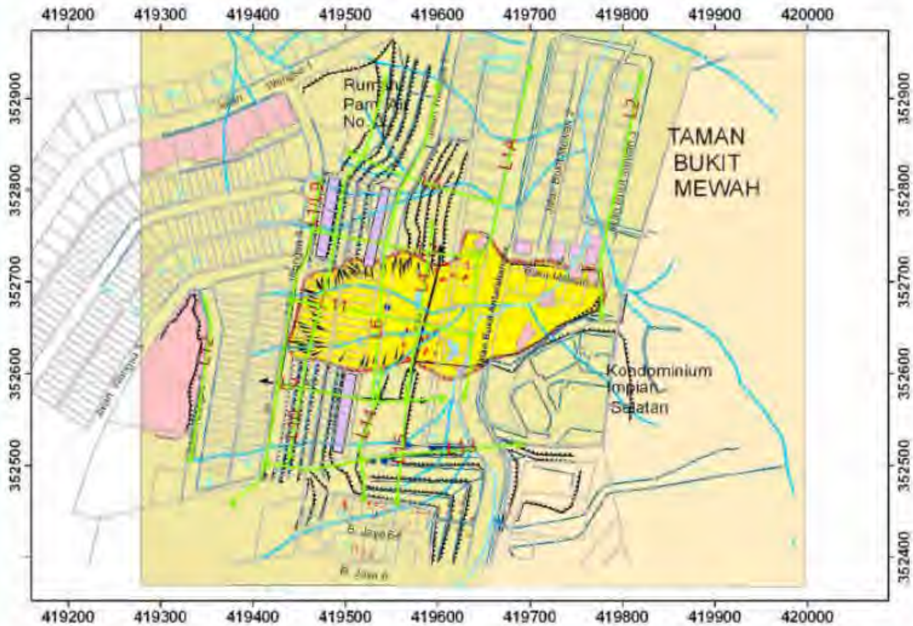
Plan View of the Geophysical Survey Lines
