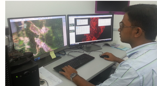
Stereo digitizing using DPW
