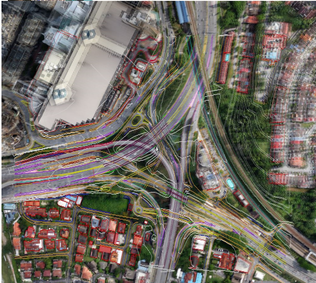
Stereo digitizing using DPW
