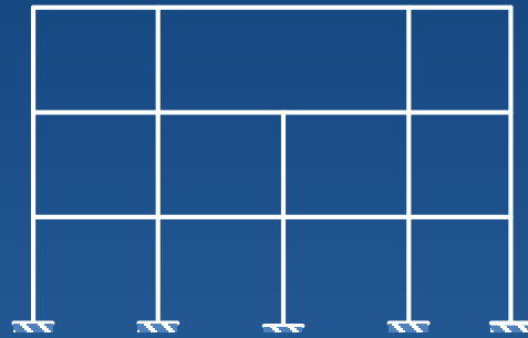
Reduced number of columns at upper floors
