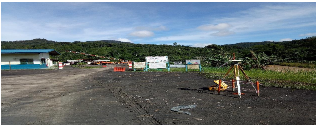
GPS Base Station 2 (E2641087.041, N5482587.465 H: 465.004m)
