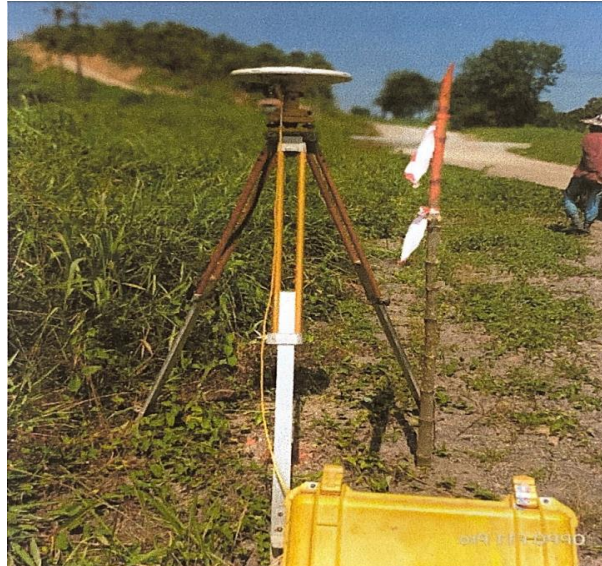
GPS Base Station 1 (E2635078.964, N5514580.808 H: 632.134m)
