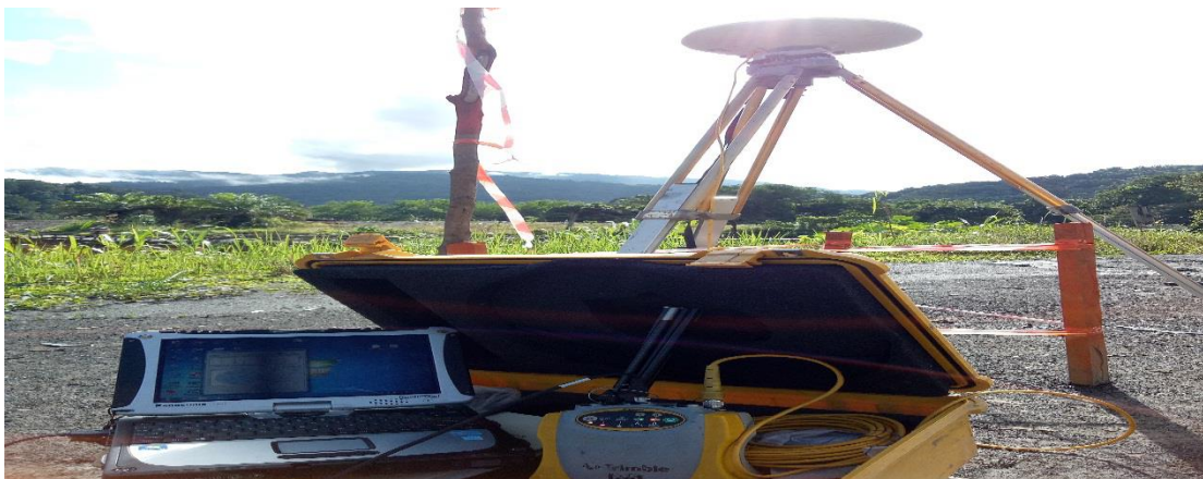
GPS base station during LiDAR flight
