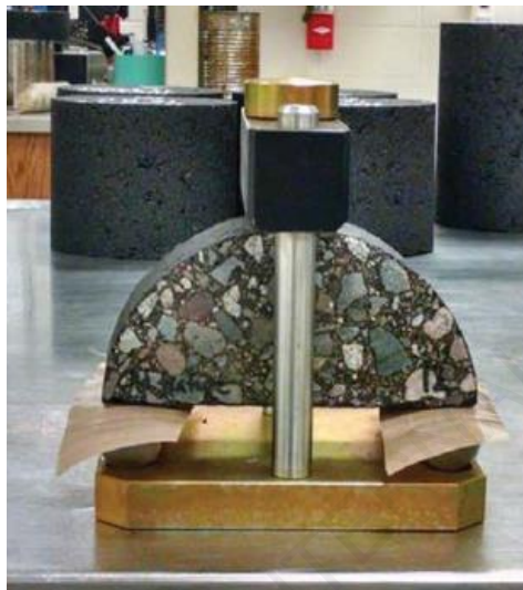
(c) Sample placed in Marshall fixture
