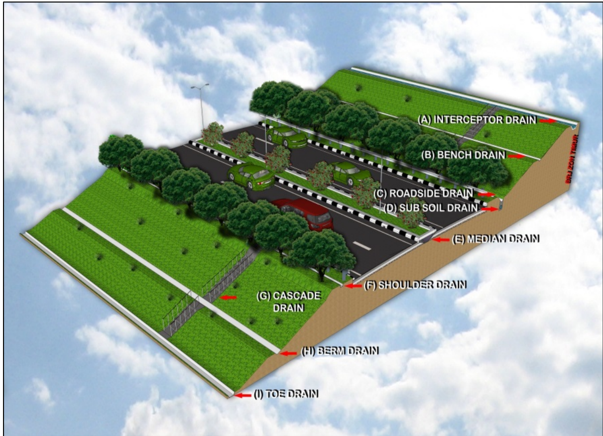
Figure 1.1 : Types of Surface Drainage
