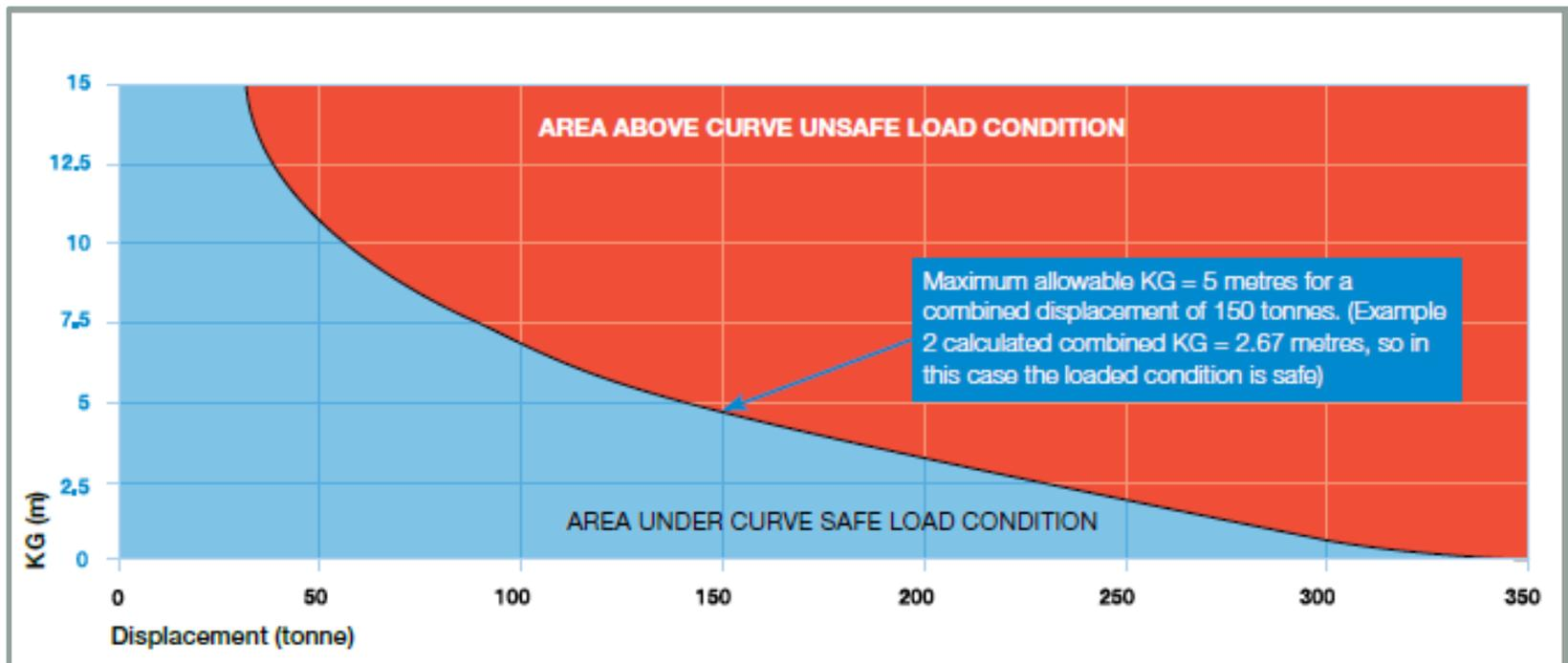
The area **under** the curve is a **safe** load condition.
