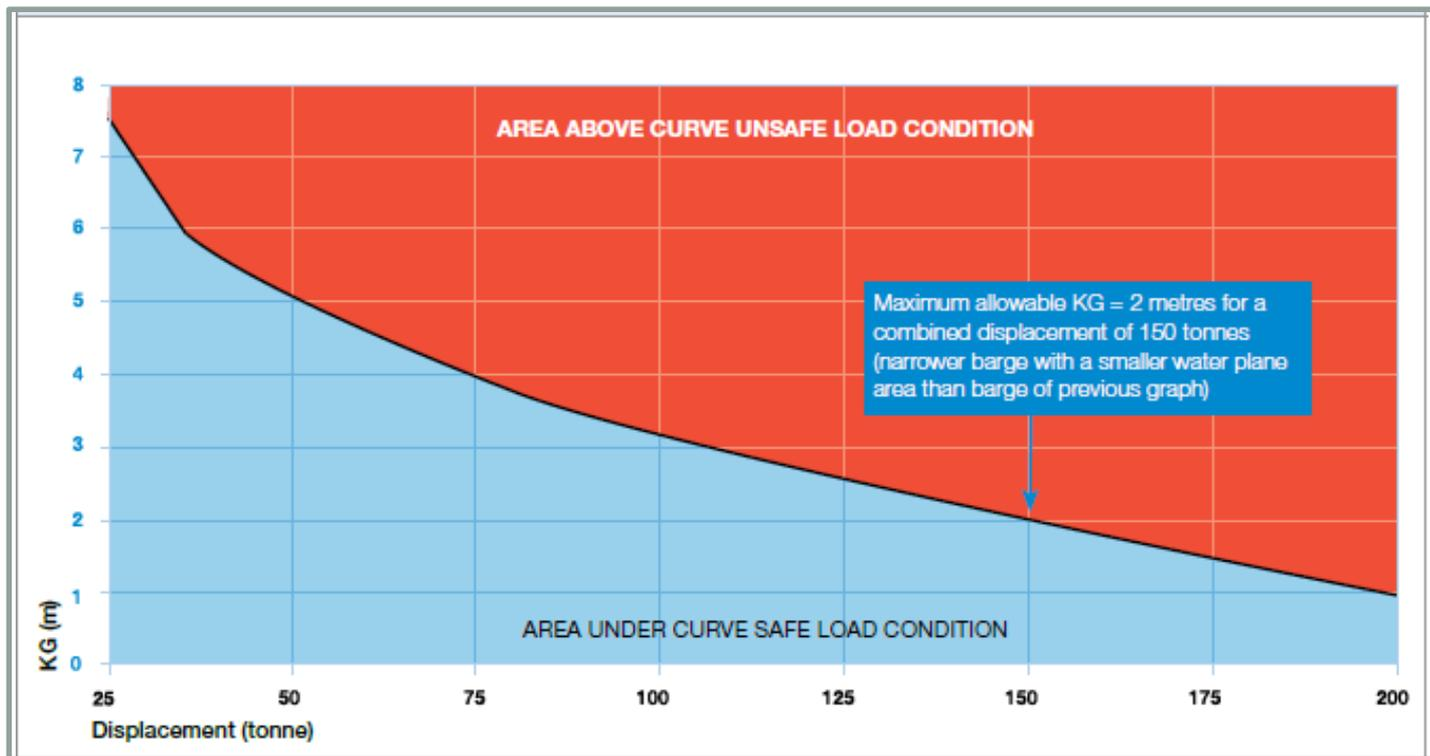
The area under the curve is a **safe** load condition.
