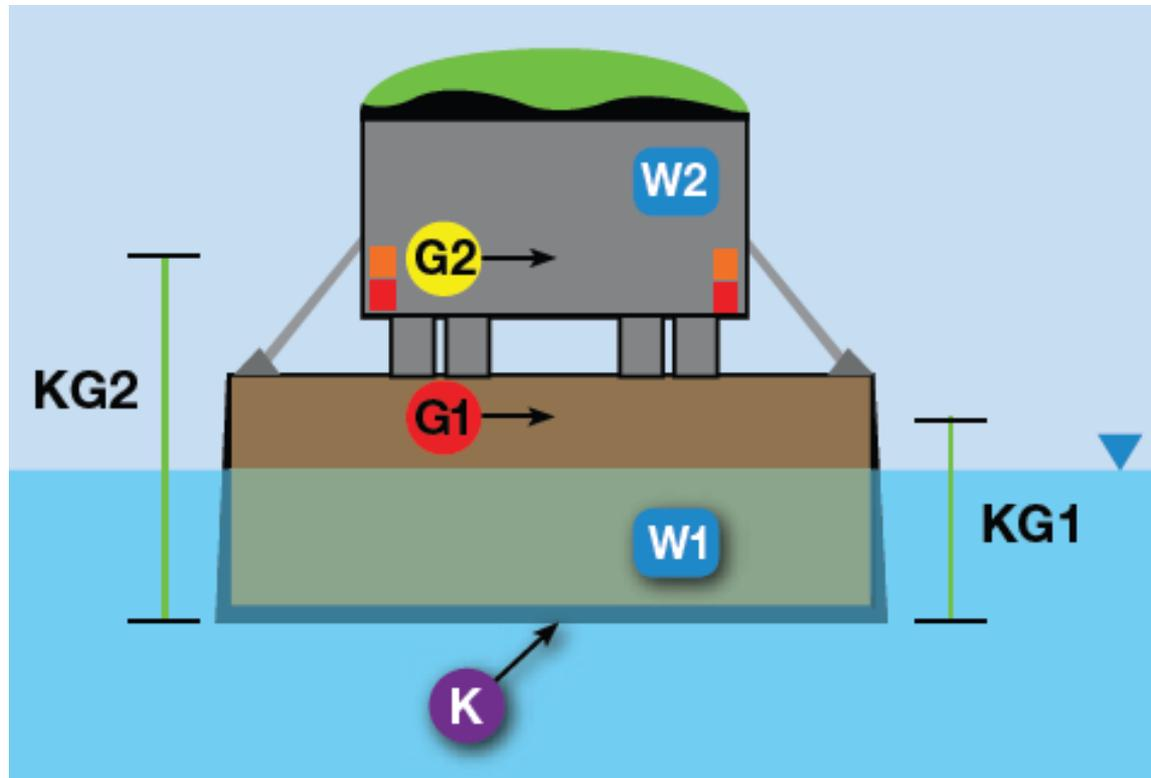
$$\text{COMBINED KG} = \frac{(\text{KG1} \times \text{W1}) + (\text{KG2} \times \text{W2})}{(\text{W1} + \text{W2})}$$
