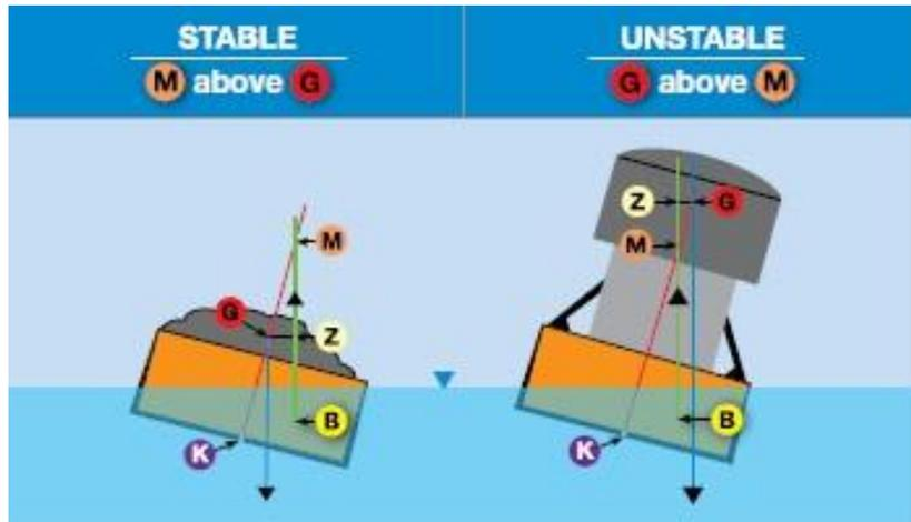
Metacentric height (GM) - the vertical distance between the Centre of Gravity (G) and the Metacentre (M). If M is above G the vessel will want to stay upright and if G is above M the vessel will want to capsize. i.e. GM positive is Stable, GM negative is Unstable.
