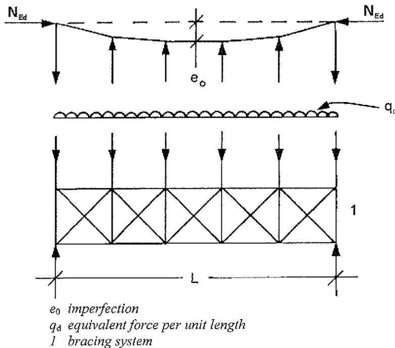
The force  $N_{Ed}$  is assumed uniform within the span  $L$  of the bracing system. For non-uniform forces this is slightly conservative.
