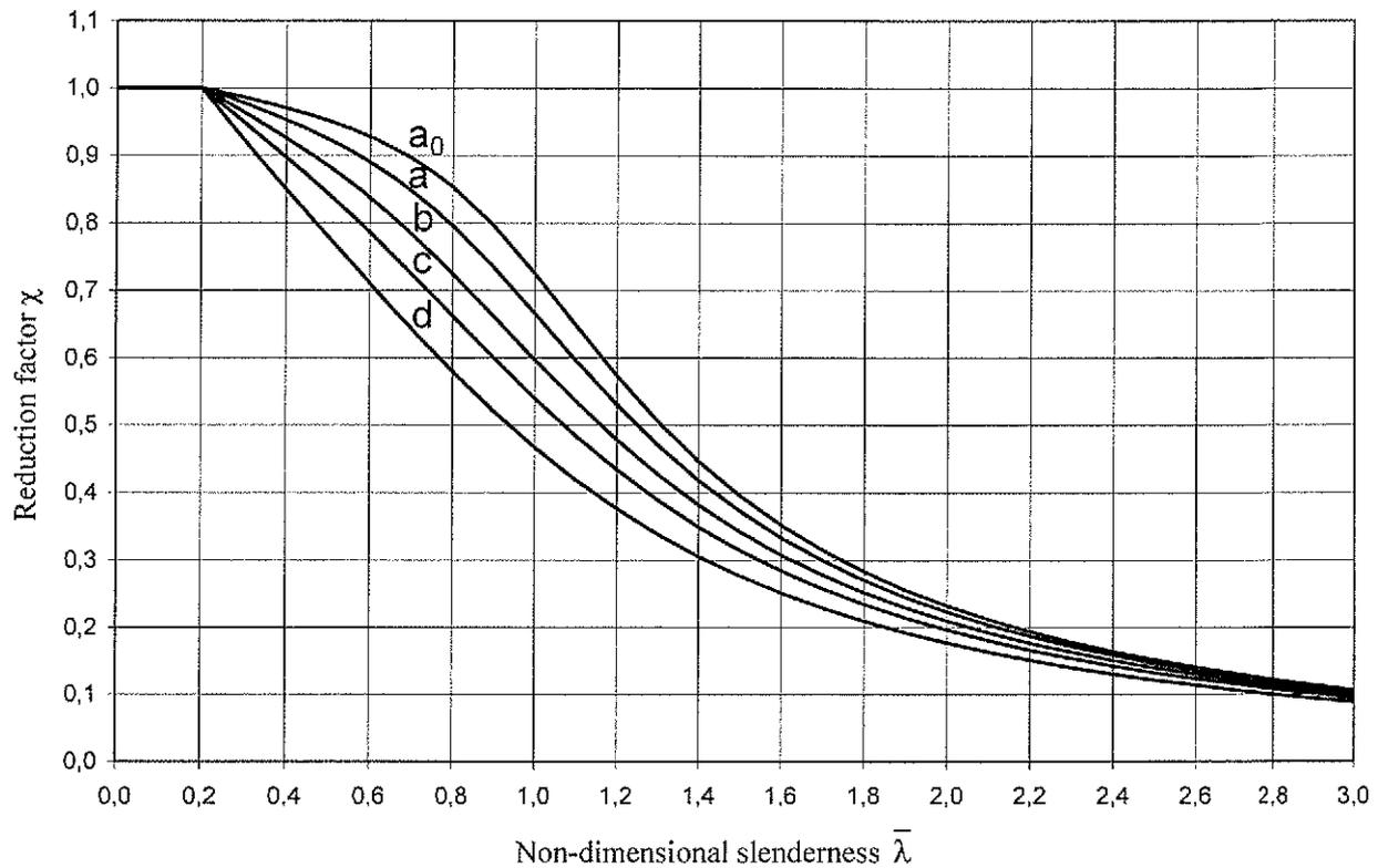
Figure 6.4: Buckling curves
