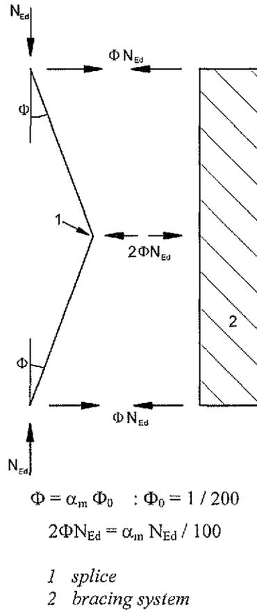
**Figure 5.7: Bracing forces at splices in compression elements**
