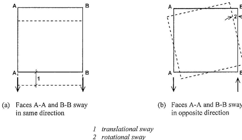
**Figure 5.5: Translational and torsional effects (plan view)**
