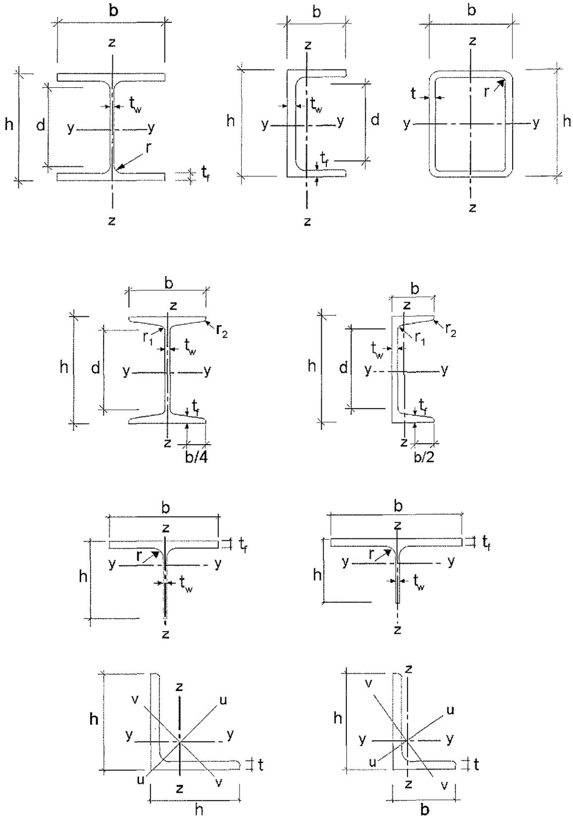
Figure 1.1: Dimensions and axes of sections
