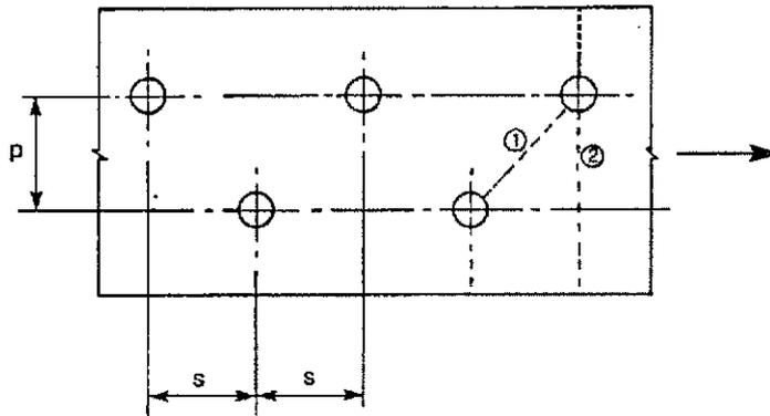
Figure 6.1: Staggered holes and critical fracture lines 1 and 2
