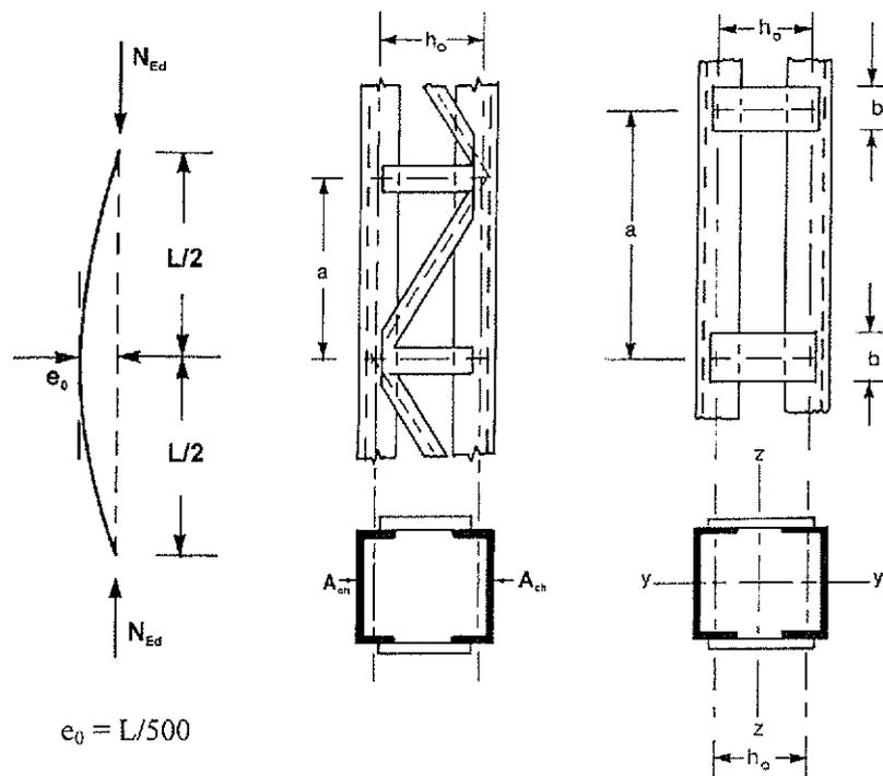
Figure 6.7: Uniform built-up columns with lacings and battening
