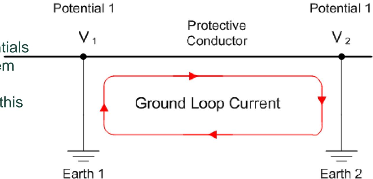
**Ground loops can be undesirable because they create a path for noise currents to flow**
