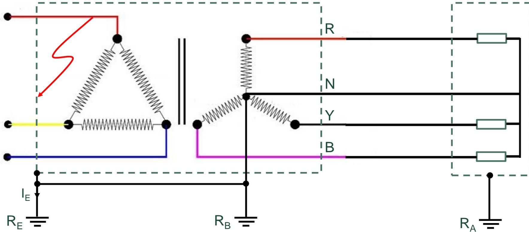
$R_E$  and  $R_B$  connected: Voltage RE, YE, BE @ MSB =  $R_E \times I_E + 230$
