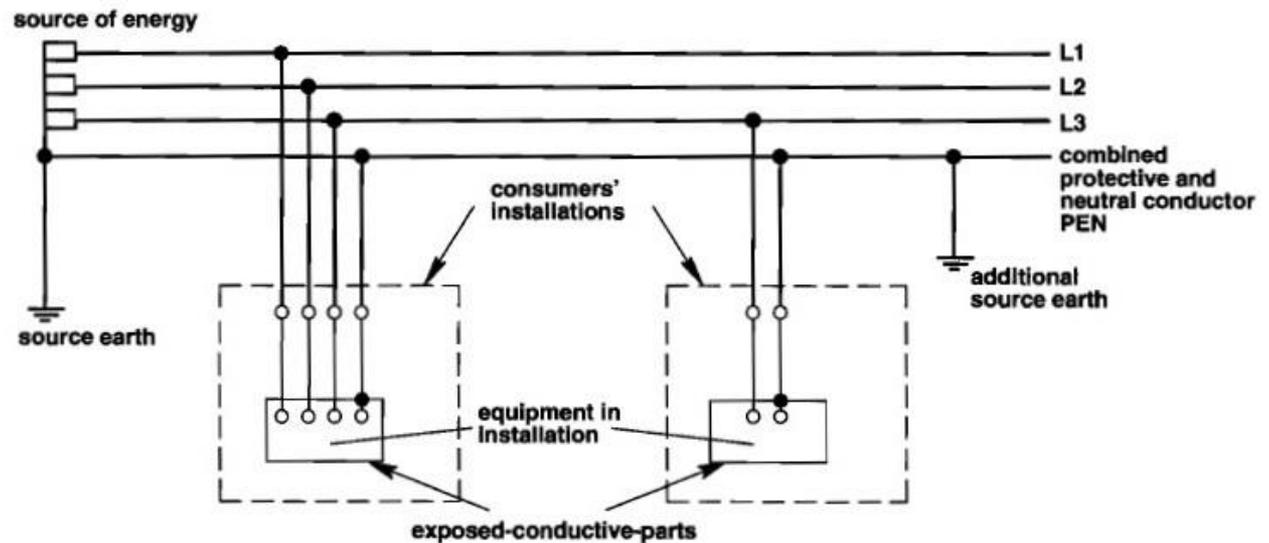
Neutral and protective functions combined in a single conductor throughout system.
