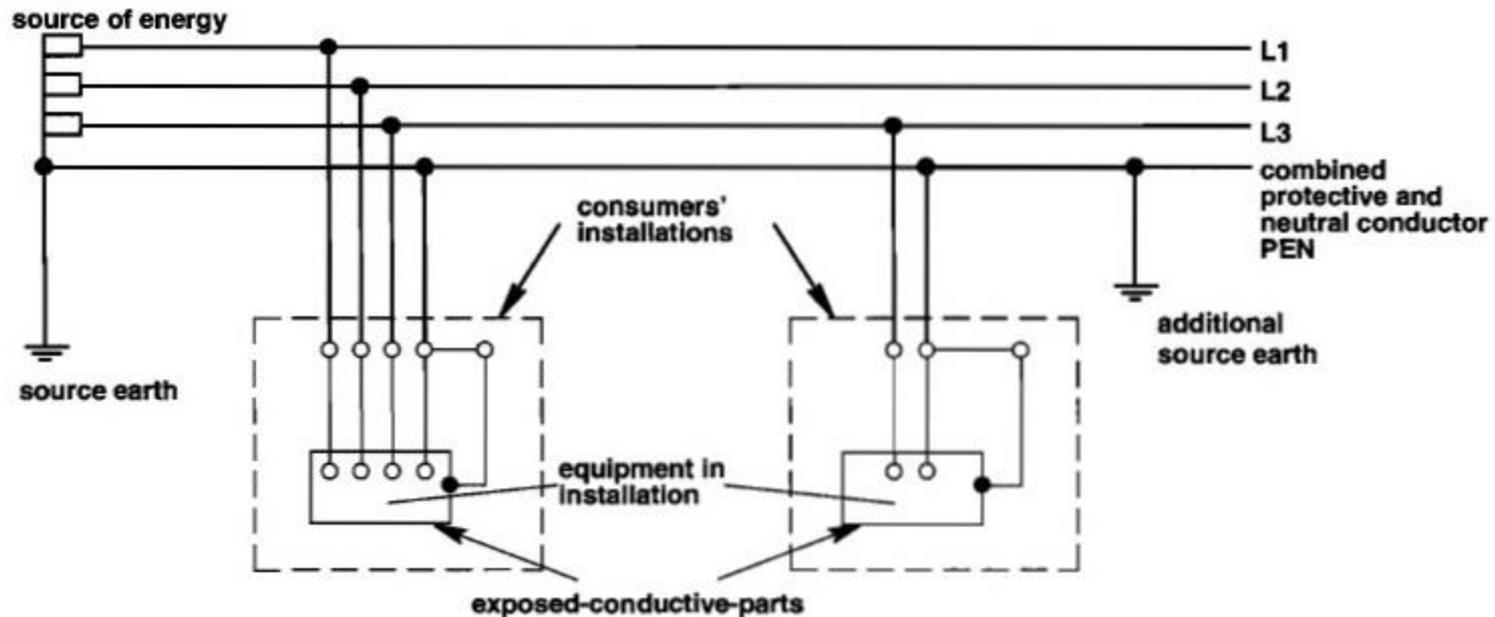
Neutral and protective functions combined in a single conductor in a part of the system.
