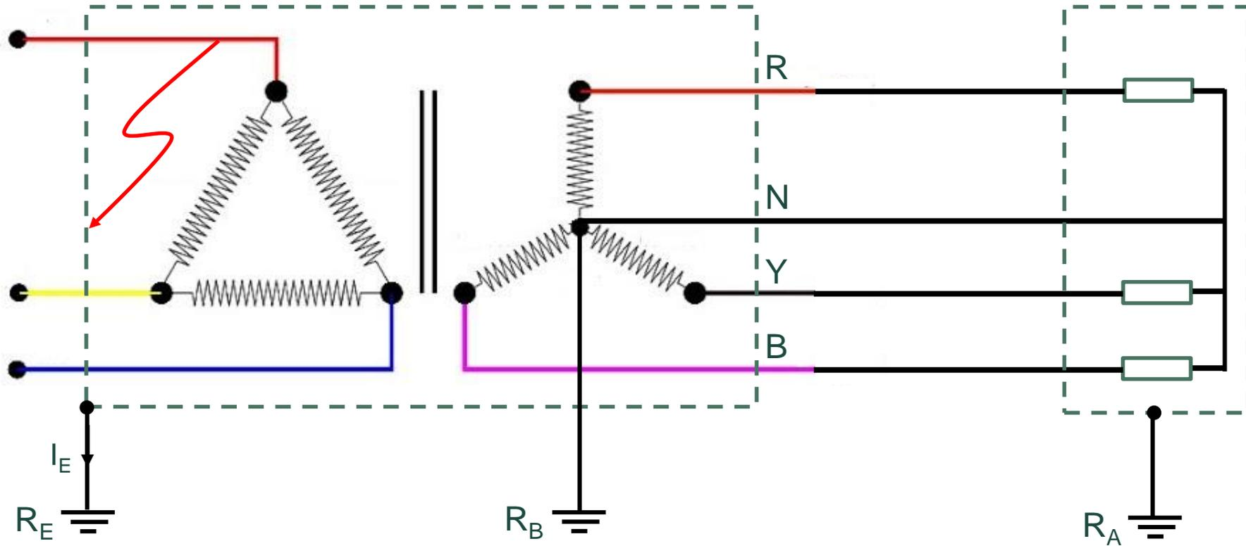
$R_E$  and  $R_B$  separated: Voltage RE, YE, BE @ MSB = 230 V
