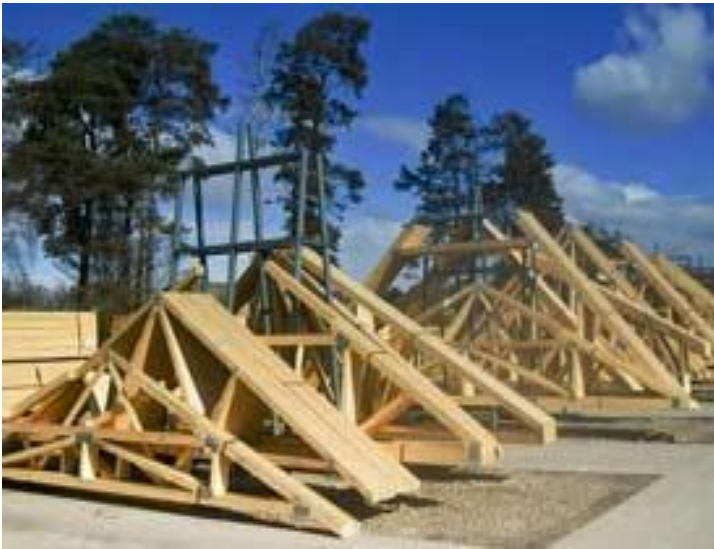
Fabricated timber trusses
