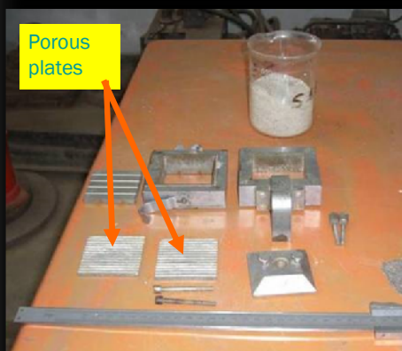
Components of the shear box
