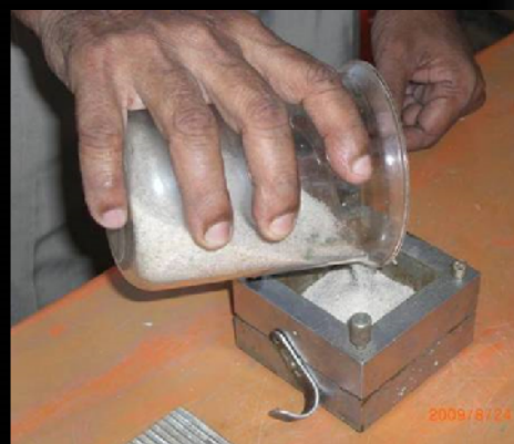
Preparation of a sand specimen
