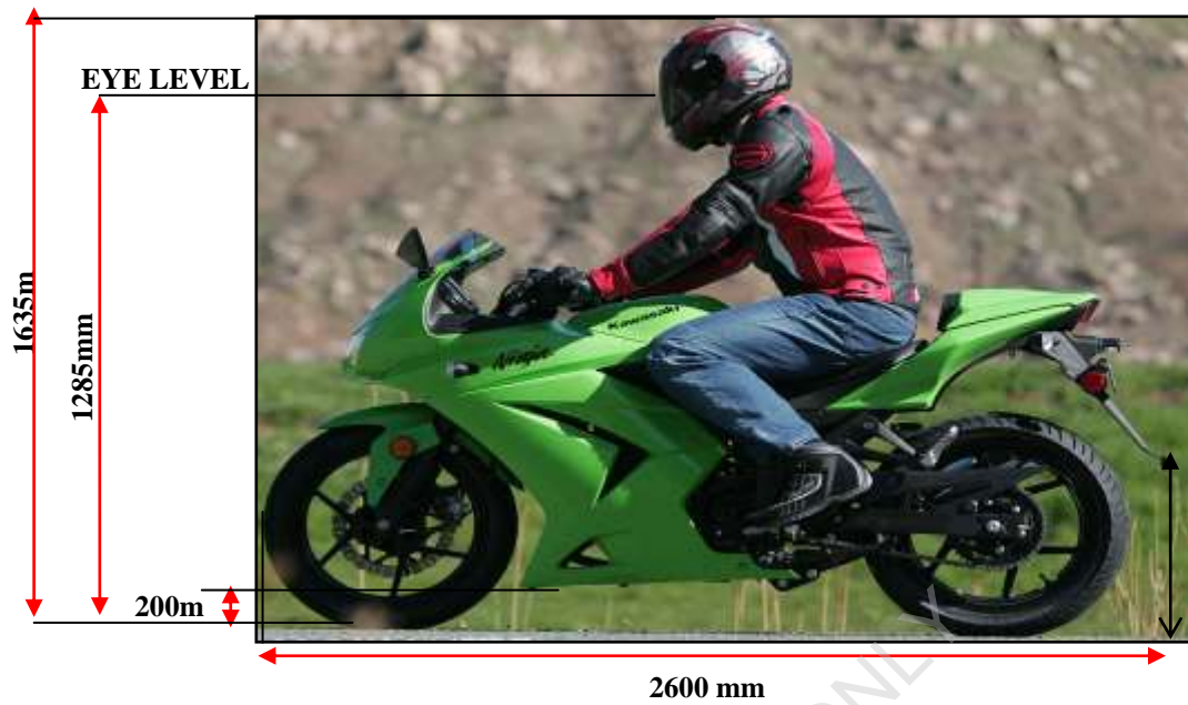
Figure 3.4: Side Outline of a Static Motorcyclist – Length of 2.60 m
