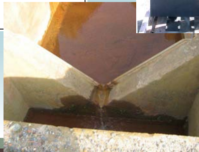
Flow Through a V-Notch Weir
