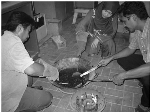
Bancuhan aggregate & bitumen (asphalt)
