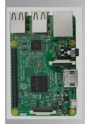
Raspberry Pi 3: 3.3 V, 900 MHz, Wifi, microSD, Ethernet, network capable, nonvolatile storage, Serial IO, GNU Linux OS
