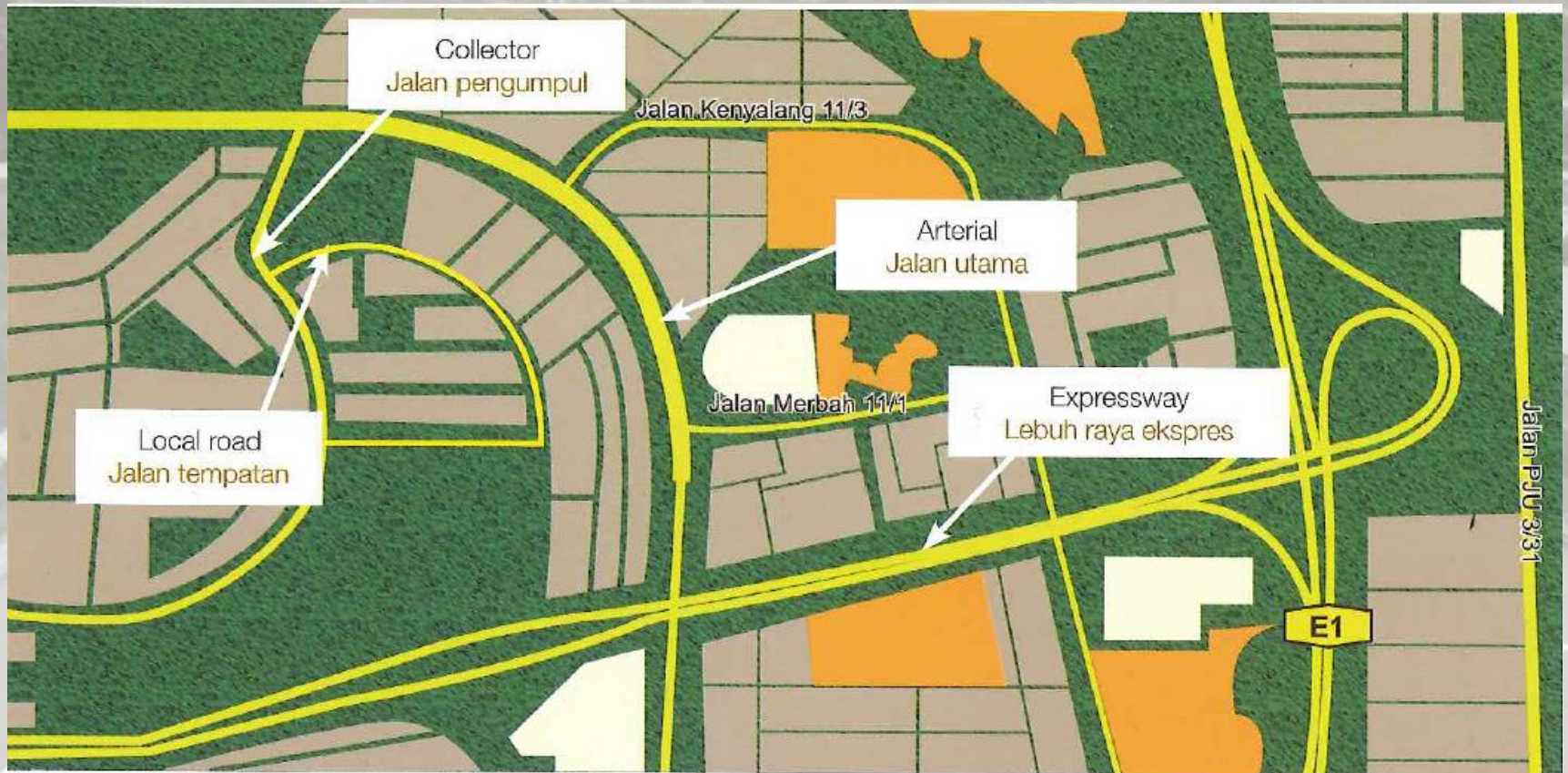
Typical Road Links in Urban Area
