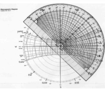
Figure 3. Superimposed shadow angle protractor on sun path diagram
