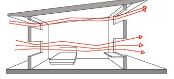
in warm climates: align window openings to user height - eg desks, seats, tables. high level openings allow night cooling of thermal mass
