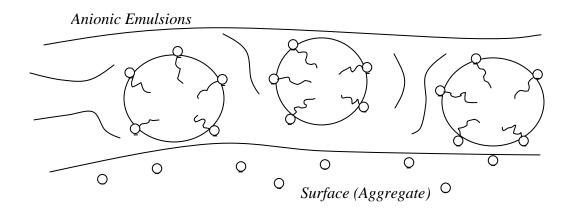
In an application of cationic emulsion, we are applying positively charged drops of asphalt to a negatively charged surface. The asphalt drops are immediately attracted to the surface and begin to break. The emulsion also losses water by evaporation. Thus the cationic emulsion has two breaking mechanisms at work and will break faster than a corresponding anionic emulsion. A depiction of the application is shown below.
