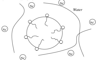
Droplet has a Net Negative Charge.
