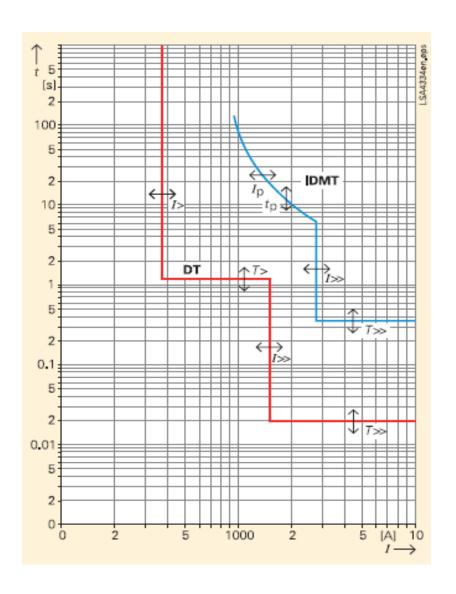
Figure shows the basic characteristics of definite and inverse-time overcurrent protection.
